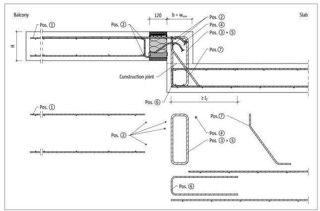
Fig. 113: Schöck Isokorb<sup>®</sup> XT type K-O: On-site reinforcement for balcony with height offset upwards with minimum structural element dimension ( $w_{vorh} = w_{min}$ )
