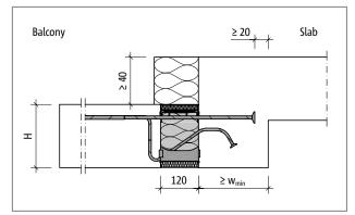
Fig. 4: Schöck Isokorb® XT type K-U with REI120: Fire protection board top and bottom; laterally integrated fire protection strips
