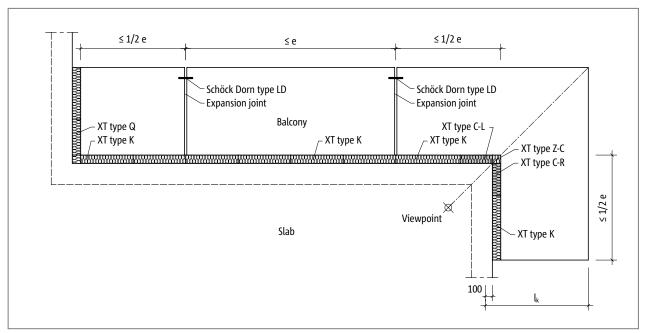
Fig. 63: Schöck Isokorb® XT type C: Expansion joint arrangement
