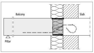
Fig. 199: Schöck Isokorb® XT type Z, Q: Thermal insulating composite system (TICS)
