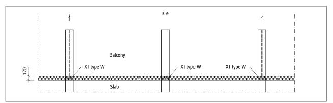
Fig. 272: Schöck Isokorb® XT type W: Expansion joint arrangement
