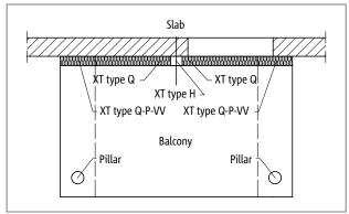
Fig. 153: Schöck Isokorb<sup>®</sup> XT type Q-P-VV, Q: Balcony with column support with various bearing stiffnesses; optionally with XT type H for transmission of ordinary horizontal force
