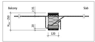
Fig. 33: Schöck Isokorb® XT type K-M7 to M10: Product section
