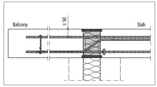
Fig. 57: Schöck Isokorb® XT type C-CV35: Connection with non-load-bearing cavity wall masonry
