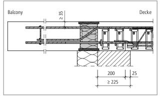
Fig. 74: Schöck Isokorb® XT type C: Prefabricated slab without edge support with TICS (section XT type C-L-CV35, view XT type C-R-CV50)
