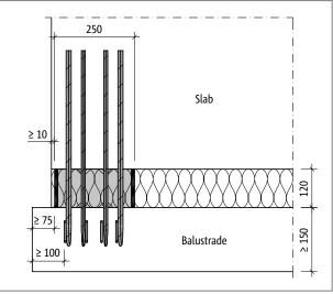
Fig. 241: Schöck Isokorb® XT type F: Top view edge distances
