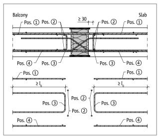
Fig. 213: Schöck Isokorb® XT type D: On-site reinforcement
