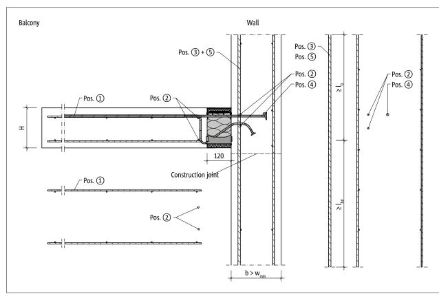
Fig. 112: Schöck Isokorb® XT type K-U: On-site reinforcement for wall connection upwards with larger structural element dimension (w<sub>varh</sub> > w<sub>min</sub>)
