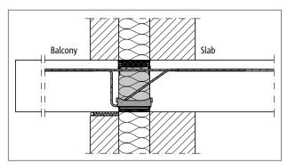
Fig. 25: Schöck Isokorb $^{\otimes}$  XT type K: Cavity wall with a balcony at inner slab level
