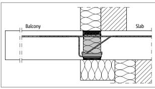
Fig. 24: Schöck Isokorb® XT type K: Connection for indirectlypositioned floor and TICS
