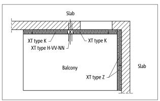
Fig. 172: Schöck Isokorb® XT type H: Balcony freely cantilevered
