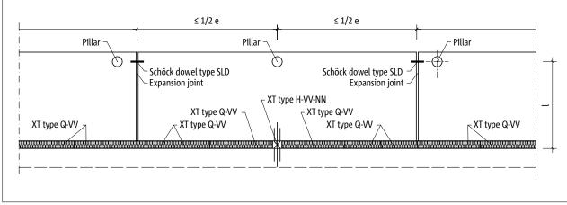
Fig. 179: Schöck Isokorb® XT type H: Expansion joint arrangement
