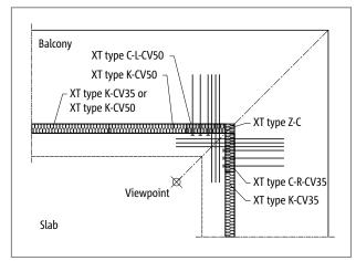
Fig. 54: Schöck Isokorb<sup>®</sup> XT type C: Balcony with outer corner freely cantilevered (applicationf XT type C-L-CV50, XT type C-R-CV35)
