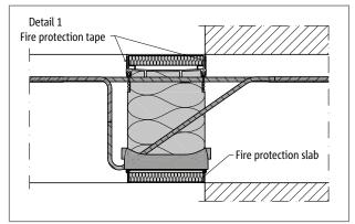
Fig. 2: Schöck Isokorb® XT type K with REI120: Detail 1
