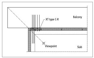
Fig. 56: Schöck Isokorb® XT type C: Balcony projecting over corner of building (application XT type C-R)
