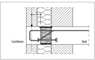
Fig. 246: Schöck Isokorb® XT type O: Corbel with faced masonry
