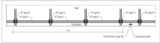
Fig. 250: Schöck Isokorb® XT type O: Expansion joint arrangement
