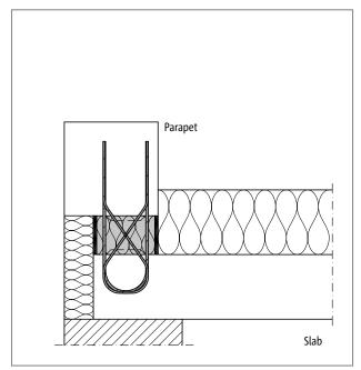
Fig. 216: Schöck Isokorb® XT type A: Connection of a parapet (XT type A-MM1)
