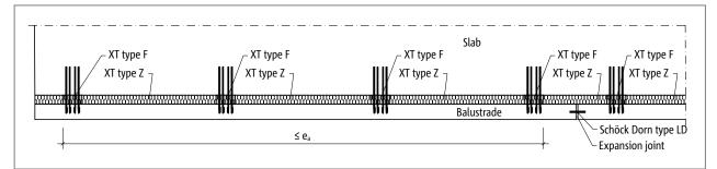
Fig. 240: Schöck Isokorb® XT type F: Expansion joint arrangement
