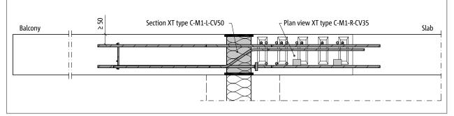
Fig. 60: Schöck Isokorb® XT type C: Outer corner with non-load-bearing cavity wall masonry (view XT type C-L-CV50; section XT type C-R-CV35)
