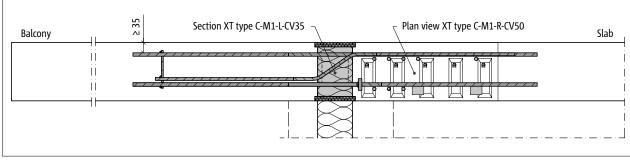
Fig. 59: Schöck Isokorb® XT type C: Outer corner with non-load-bearing cavity wall masonry (section XT type C-L-CV35; view XT type C-R-CV50)
