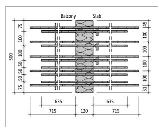
Fig. 69: Schöck Isokorb<sup>®</sup> XT type C-R-M2-V2: Product plan view
