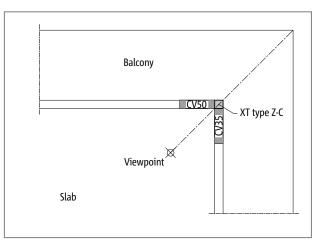
Fig. 50: Schöck Isokorb® XT type C: Concrete cover selectable: Here CV50 left from viewpoint, concrete cover CV35 right from viewpoint
