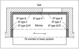
Fig. 152: Schöck Isokorb® XT type Q, Q-PZ: Recessed balcony, supported on three sides - symmetric with tie member
