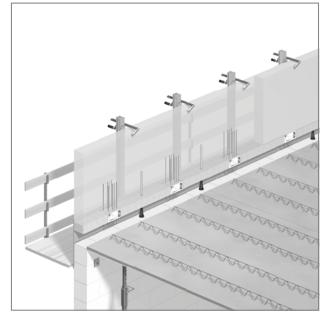
Fig. 234: Schöck Isokorb® XT type A with Combar® FT erection support: Securing of the aligned precast concrete parapet
