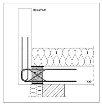
Fig. 236: Schöck Isokorb® XT type F: Connection of a frontally attached balustrade with thermal insulation composite system (TICS))
