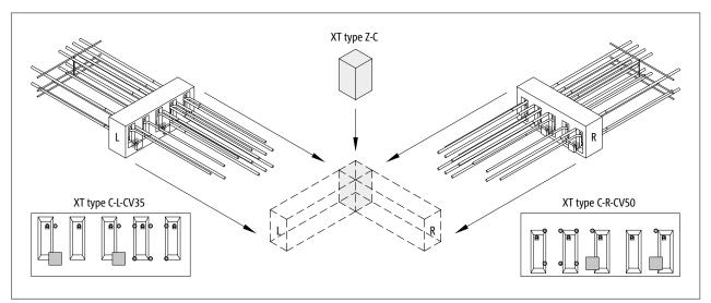
Fig. 51: Schöck Isokorb® XT type C-L-CV35, XT type C-R-CV50: Arrangement at the corner using corner insulating element
