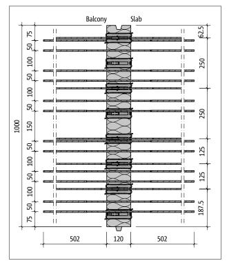
Fig. 31: Schöck Isokorb® XT type K-M4: Product plan view
