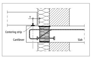
Fig. 247: Schöck Isokorb® XT type O: Connection of a console as floor support; centring battens prevent a displacement of the load application point
