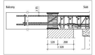
Fig. 76: Schöck Isokorb® XT type C: Prefabricated slab with edge support with thermal insulating masonry (section XT type C-L-CV35, view XT type C-R-CV50)
