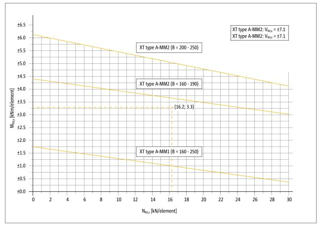
The point (( $N_{Ed,z}$ ;  $M_{Ed,y}$ ) = (16.2 kN; 3.3 kNm) lies below the line of the Schöck Isokorb<sup>®</sup> XT type A-MM2 (B = 200 - 250). Thus the verification is rendered.
