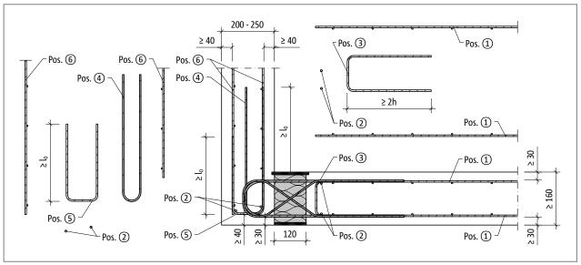
Fig. 244: Schöck Isokorb<sup>®</sup> XT type F: On-site reinforcement with parapet/balustrade width b = 200 - 250; on-site reinforcement b = 160 - 190 such as b = 200 - 250 without Pos. 5
