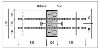
Fig. 162: Schöck Isokorb® XT type Q-P-VV1: Product plan view
