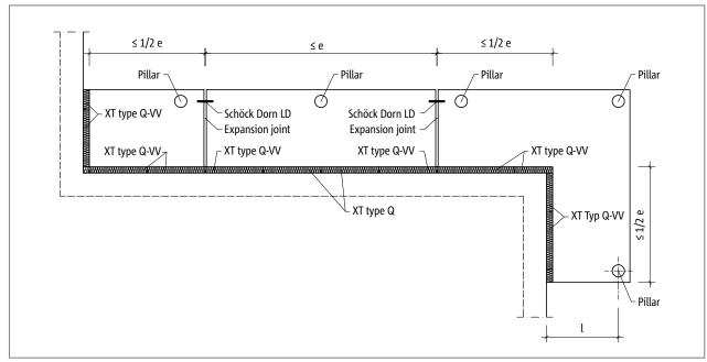
Fig. 133: Schöck Isokorb® XT type Q, Q-VV: Expansion joint arrangement
