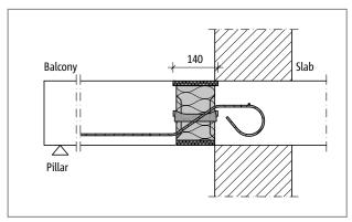
Fig. 3: Schöck Isokorb® XT type Q with REI120: Fire protection board top projecting laterally
