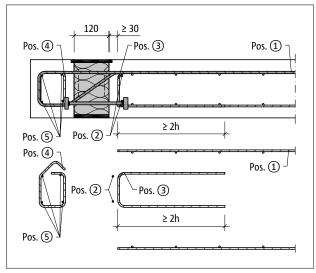
Fig. 254: Schöck Isokorb® XT type O: On-site reinforcement
