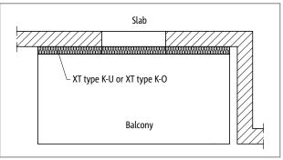
Fig. 86: Schöck Isokorb® XT type K-U/K-O: Balcony with facade offset
