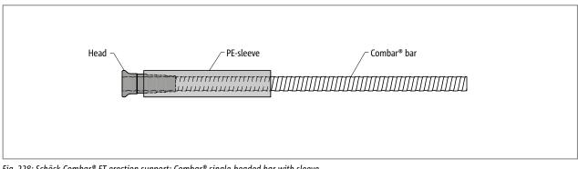
Fig. 228: Schöck Combar® FT erection support: Combar® single-headed bar with sleeve
