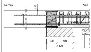
Fig. 77: Schöck Isokorb<sup>®</sup> XT type C: Prefabricated slab with edge support with thermal insulating masonry (section XT type C-R-CV50, view XT type C-L-CV35)
