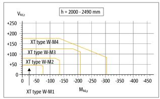
Fig. 271: Schöck Isokorb® XT type W: Interaction diagram
