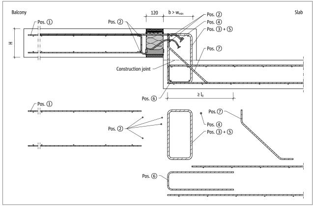
Fig. 114: Schöck Isokorb® XT type K-O: On-site reinforcement for balcony with height offset upwards with larger structural element dimension (w<sub>vorh</sub> > w<sub>min</sub>)
