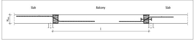
Fig. 156: Schöck Isokorb® XT type Q-PZ, Q-P: Static system
