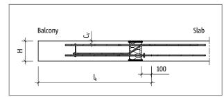
Fig. 62: Schöck Isokorb® XT type C: Static system
