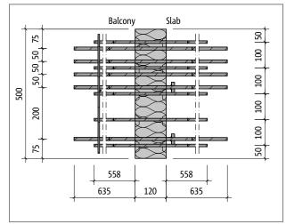
Fig. 66: Schöck Isokorb® XT type C-L-M1-V1: Product plan view
