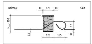
Fig. 138: Schöck Isokorb® XT type Q-Z-V1 to Q-Z-V4: Product section
