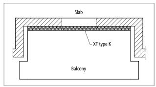
Fig. 20: Schöck Isokorb® XT type K: Balcony with facade recess
