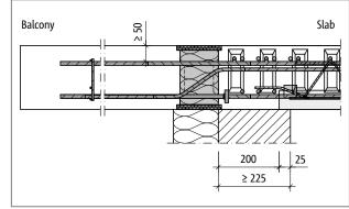
Fig. 75: Schöck Isokorb® XT type C: Prefabricated slab without edge support with TICS (section XT type C-R-CV50, view XT type C-L-CV35)
