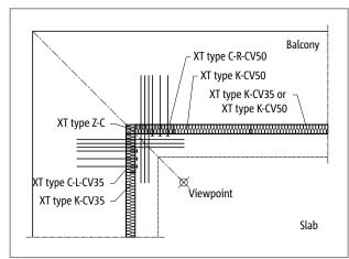
Fig. 53: Schöck Isokorb® XT type C: Balcony with outer corner freely cantilevered (application XT type C-L-CV35, XT type C-R-CV50)
