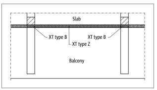
Fig. 257: Schöck Isokorb® XT type B: Balcony construction with freely cantilevered downstand beams
