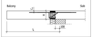
Fig. 26: Schöck Isokorb® XT type K: Static system
