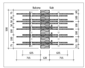
Fig. 68: Schöck Isokorb® XT type C-L-M2-V2: Product plan view
