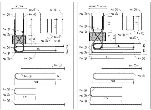
Fig. 227: Schöck Isokorb® XT type A: On-site reinforcement on the inside (B = 160 and B = 200)
