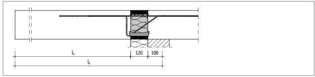
Fig. 9: Schöck Isokorb<sup>®</sup> XT type K: System cantilever length  $(l_k)$  for design and geometric cantilever  $(l_b)$
