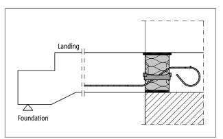
Fig. 126: Schöck Isokorb® XT type Q: Connection stair landing with single wall thermally insulating masonry (XT type Q-V1 to V4)
