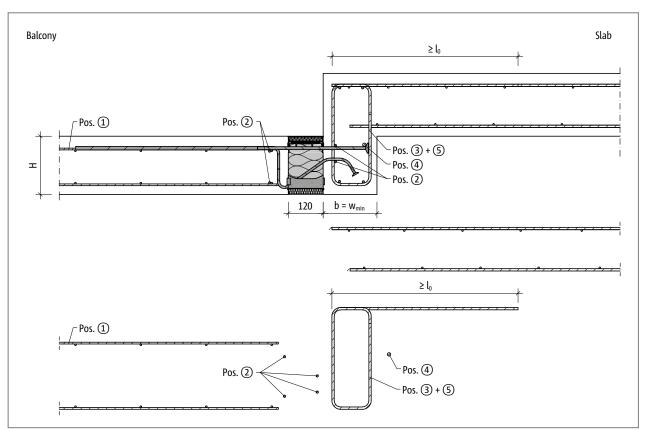
Fig. 109: Schöck Isokorb<sup>®</sup> XT type K-U: On-site reinforcement for balcony with height offset downwards with minimum structural element dimension ( $w_{vorh} = w_{min}$ )
