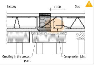
Fig. 43: Schöck Isokorb® XT type K: Direct support, installation in conjunction with element slabs (here:  $h \le 180$  mm), compression joint on floor side
