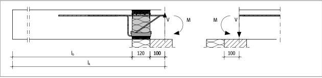
Fig. 11: Schöck Isokorb® XT type K: Determined design stress resultants applied to floor slab
