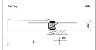
Fig. 46: Schöck Isokorb® XT type K: Static system
