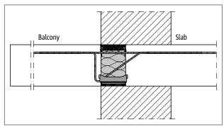
Fig. 23: Schöck Isokorb® XT type K: Connection with single-leaf masonry
