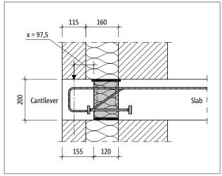
Fig. 255: Schöck Isokorb® XT type O: Wall construction for design example
