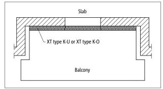
Fig. 87: Schöck Isokorb<sup>®</sup> XT type K-U/K-O: Balcony with facade offset
