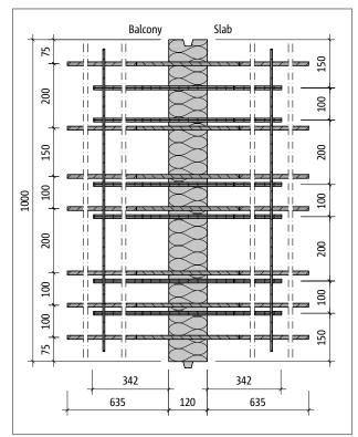
Fig. 211: Schöck Isokorb® XT type D-MM3-VV1: Plan view
