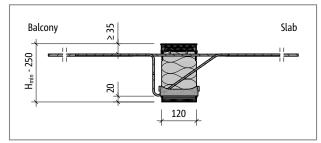
Fig. 29: Schöck Isokorb® XT type K-M1 to M4: Product section
