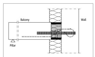
Fig. 176: Schöck Isokorb® XT type Q, H-VV-NN: Connection to a reinforced concrete wall with external insulation
