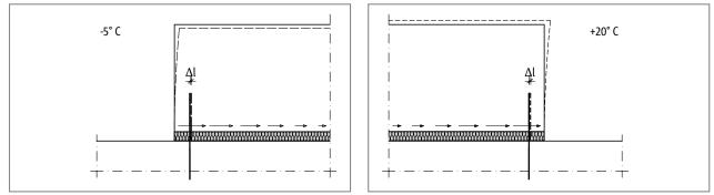
Fig. 13: Schöck Isokorb<sup>®</sup>: Displacement of the outer bars of a balcony slab by  $\Delta I$  as a result of temperature deformation
