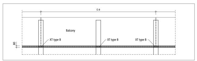
Fig. 261: Schöck Isokorb® XT type B: Expansion joint arrangement
