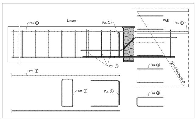
Fig. 265: Schöck Isokorb® XT type B: On-site reinforcement
