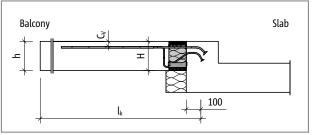
Fig. 98: Schöck Isokorb® XT type K-O: Static system
