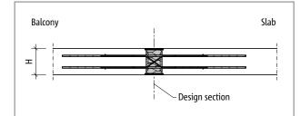
Fig. 208: Schöck Isokorb® XT type D: Static system
