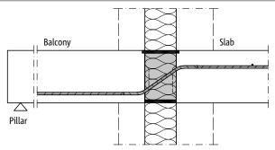
Fig. 122: Schöck Isokorb® XT type Q: Connection with non-load-bearing dou-
