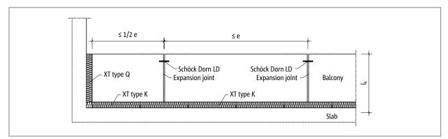
Fig. 28: Schöck Isokorb® XT type K: Expansion joint arrangement
