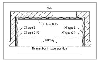
Fig. 151: Schöck Isokorb® XT type Q-VV, Q-P, Q-PZ: Recessed balcony, supported on three sides with tie member
