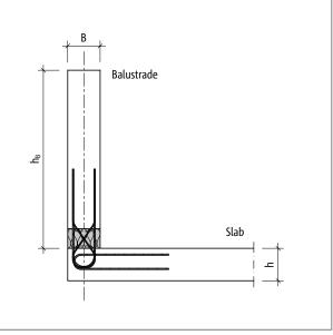
Fig. 219: Schöck Isokorb® XT type A: Static system
