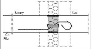
Fig. 121: Schöck Isokorb® XT type Q: Connection with non-load-bearing double wall masonry (XT type Q-V1 to V4)
