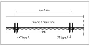
Fig. 220: Schöck Isokorb® XT type A: Verification met if selected distance  $a_{prov} \leq a_{max}$
