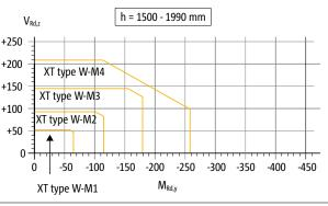
Fig. 269: Schöck Isokorb® XT type W: Interaction diagram
