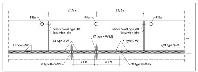
Fig. 181: Schöck Isokorb® XT type H: Expansion joint arrangement
