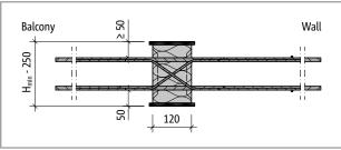
Fig. 210: Schöck Isokorb® XT type D with CV50: Product section
