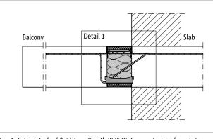
Fig. 1: Schöck Isokorb® XT type K with REI120: Fire protection boards top and bottom; laterally integrated fire protection strips
