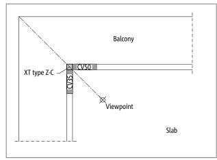
Fig. 49: Schöck Isokorb<sup>®</sup> XT type C: Concrete cover selectable: Here CV35 left from viewpoint, concrete cover CV50 right from viewpoint
