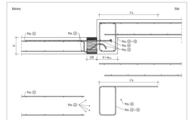
Fig. 110: Schöck Isokorb<sup>®</sup> XT type K-U: On-site reinforcement for balcony with height offset downwards with larger structural element dimension ( $w_{vorh} > w_{min}$ )
