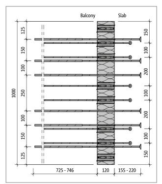
Fig. 102: Schöck Isokorb<sup>®</sup> XT type K-U-M2: Product plan view
