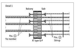
Fig. 168: Schöck Isokorb® XT type Q-P, Q-PZ: Detail 1; Reinforcement connection tie member
