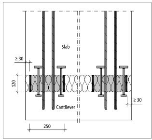
Fig. 251: Schöck Isokorb® XT type O: Edge distances to be observed
