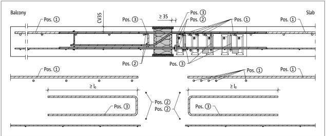
Fig. 70: Schöck Isokorb® XT type C: On-site reinforcement outer corner (section XT type C-L-CV35, view XT type C-R-CV50)
