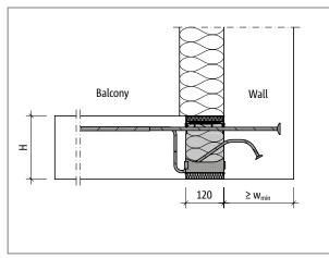
Fig. 93: Schöck Isokorb® XT type K-U: Wall connection upwards with external insulation
