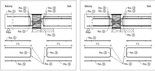
Fig. 144: Schöck Isokorb® XT type Q-V5 to Q-V8: On-site reinforcement
