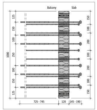
Fig. 106: Schöck Isokorb® XT type K-O-M2: Product plan view
