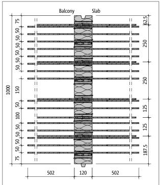
Fig. 32: Schöck Isokorb<sup>®</sup> XT type K-M6: Product plan view
