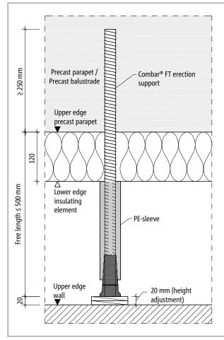
Fig. 229: Schöck Combar® FT erection support: planning dimensions
