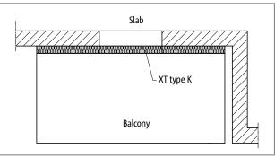
Fig. 19: Schöck Isokorb® XT type K: Balcony with facade offset
