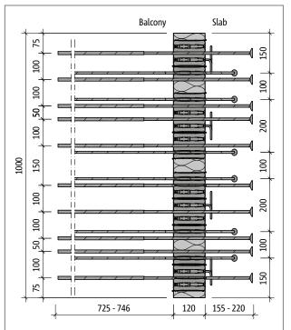
Fig. 103: Schöck Isokorb® XT type K-U-M4: Product plan view
