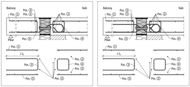
Fig. 142: Schöck Isokorb® XT type Q-V1 to V4: On-site reinforcement
