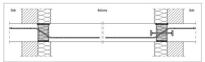
Fig. 154: Schöck Isokorb<sup>®</sup> XT type Q-P, Q-PZ: Application case recessed balcony see p. 119
