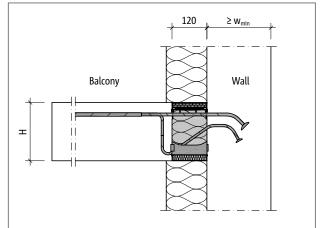
Fig. 92: Schöck Isokorb® XT type K-O: Wall connection downwards with external insulation
