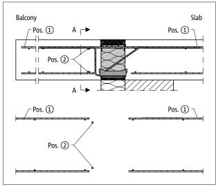
Fig. 37: Schöck Isokorb® XT type K: on-site reinforcement with direct support
