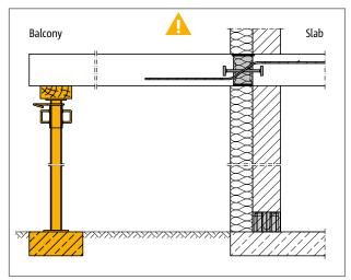
Fig. 169: Schöck Isokorb<sup>®</sup> XT type Q-P-VV: Continuous support required
