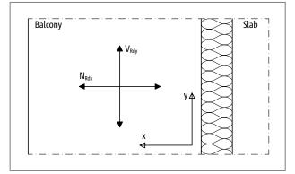
Fig. 178: Schöck Isokorb® XT type H: Sign rule for the design
