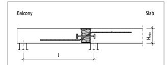
Fig. 155: Schöck Isokorb® XT type Q-P: Static system
