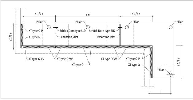
Fig. 158: Schöck Isokorb® XT type Q-P, Q-P-VV: Expansion joint arrangement
