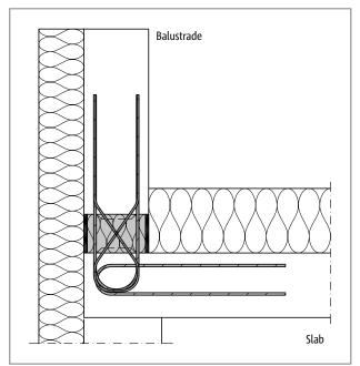
Fig. 217: Schöck Isokorb® XT type A: Connection to a balustrade (XT type A-MM2)
