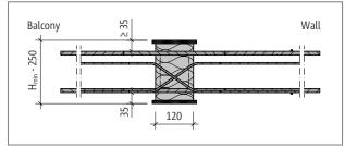
Fig. 209: Schöck Isokorb® XT type D with CV35: Product section
