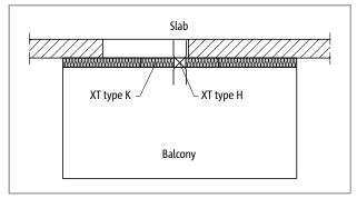
Fig. 18: Schöck Isokorb<sup>®</sup> XT type K: Balcony freely cantilevered; optional with XT type H (from page 125) with planned horizontal loads (e. g. closed ballustrades)
