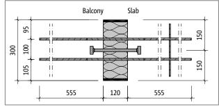
Fig. 160: Schöck Isokorb® XT type Q-P-V1: Product plan view
