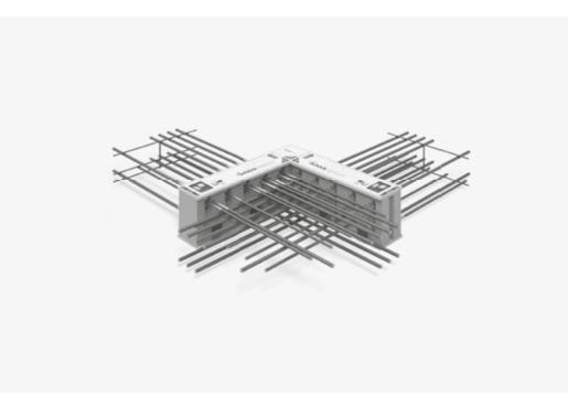
**Schöck Isokorb® XT type C** Suitable for cantilevered corner balconies. It transfers negative moments and positive shear forces.
