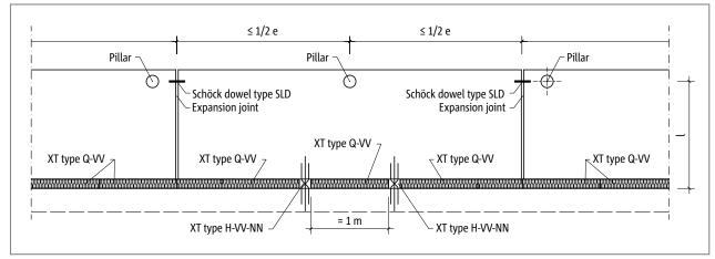
Fig. 180: Schöck Isokorb® XT type H: Expansion joint arrangement
