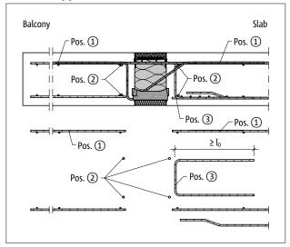
Fig. 38: Schöck Isokorb® XT type K: On-site reinforcement with indirect support
