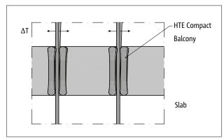
Fig. 14: Schöck Isokorb® detail: deflection of the pressure bearing as a result of temperature difference
